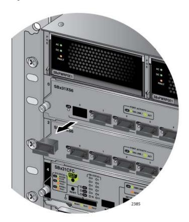
Figure 100. Removing the Dust Cover From an SFP+ Slot in the AT-SBx31XS6 Line Card
